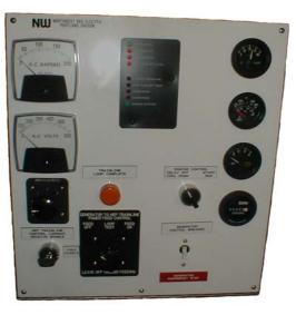
Yard Power Units: 200 (right), 400, and 800 amp units have been produced, for feeding power to cars in station or storage. Several models are available for feeding several different types of power configurations.
