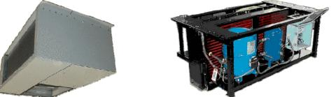
Our standard evaporator unit **(above, left)** includes blowers, heater and air conditioning evaporator that will fit in most retrofit applications. Our standard condenser **(above, right)** is built to fit most passenger cars as well. All components are constructed with railroad service in mind. For example, the condenser coil features widely spaced copper fins, so the unit will survive undercar dirt and resulting cleaning. Powder coat finish assures metal parts a long life.
