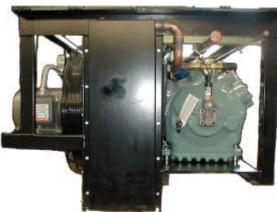
ended units. Hangers designed for support from underneath are provided at the top end of each unit. Two accurately positioned (laser-cut) holes are provided in each end for securing the frame to the hanger.
